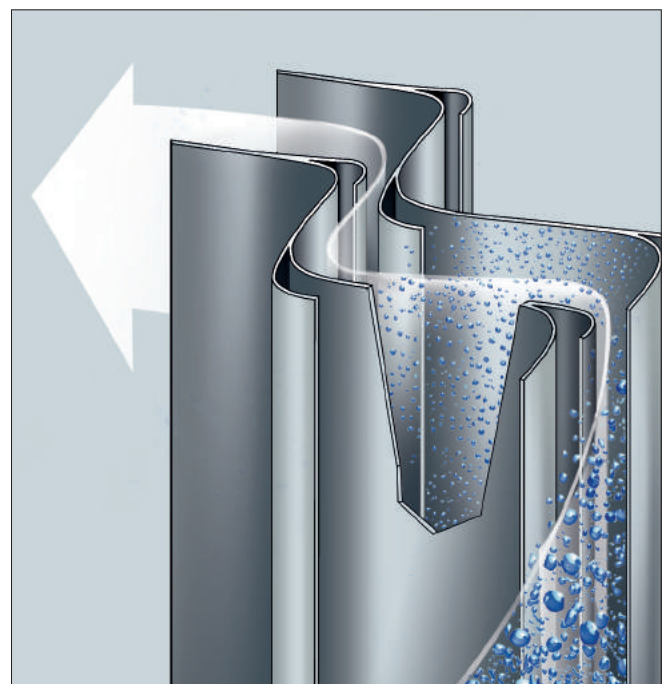
Functional principle of a horizontal separator
