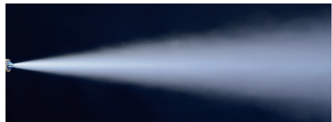
Spray pattern of a Laval nozzle
