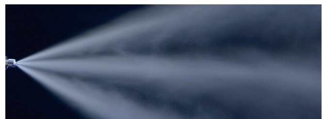
Spray pattern of a flat fan nozzle
