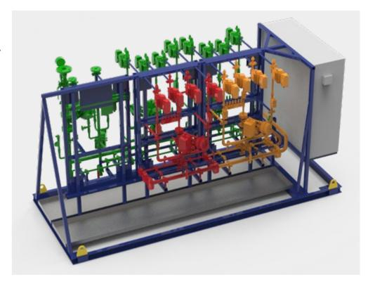
adapted. Regardless of the number of lances selected, the base frame, inlet module and control cabinet are always of the same design. Each of the identically constructed injection modules supplies two lances. The required injection modules are implemented depending on the number of lances selected. Due to the modular design, further injection modules for
