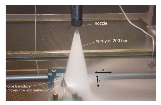
Figure 3 - Test bench to perform impact measurements
