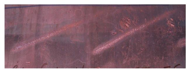
Figure 7 - No imprint on lead plate in the excessive overlap area
