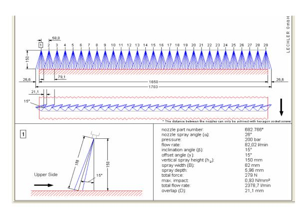
Figure 8 - Example of computer simulation with Lechler "DESCALE" program of existing situation with excessive overlap between adjacent sprays
