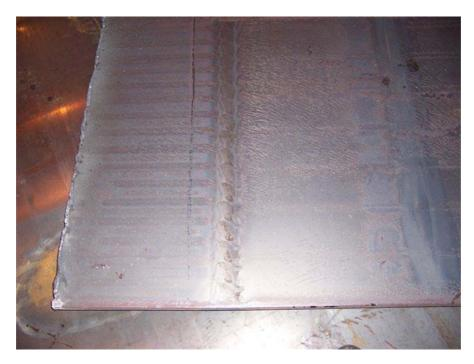
Figure 9 - Undescaled striping patterns on the surface due to non sufficient spray overlaps
