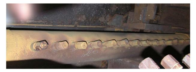
Figure 2 - Descaling header with poorly aligned nozzles
