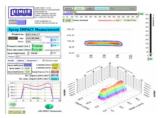
Figure 5 - Documented impact measurement of a descaling nozzle
