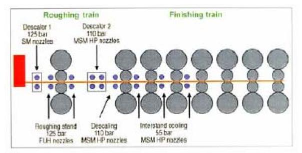
Figure 12 - TKS Bochum wide hot strip mill descaling system overview
