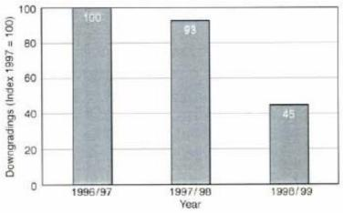
Figure 13 - Development of strip downgradings in TKS Bochum due to rolled in scale
