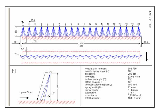
Figure 10 - Example of computer simulation with Lechler "DESCALE" program of existing situation with no overlap between adjacent sprays
