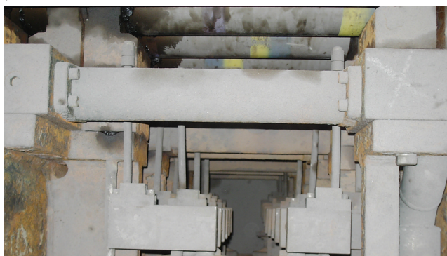
Figures 9 and 10 – “Inline” nozzle layout causing temperature striping.
