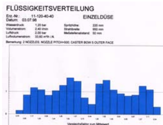
Existing cooling: Water distribution nozzle arrangements at 1,2 bar water pressure
