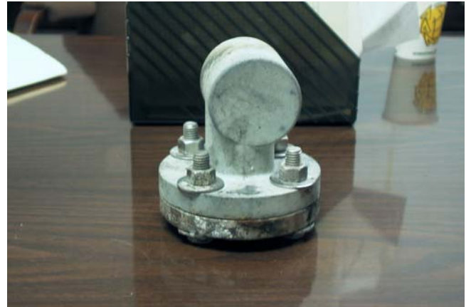
Photo 2 No erosion of ceramic nozzle after 24 weeks of service
