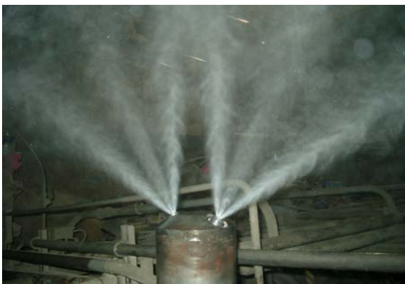
Twin-fluid Nozzle used for Semi-Dry Flue Gas Desulphurization OR Selective Catalytic Reduction
