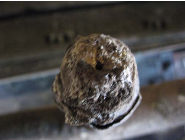
Buildup around nozzle orifice of twin-fluid nozzle
