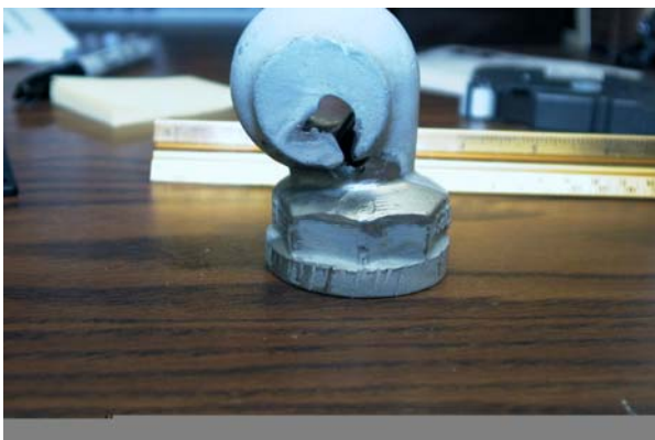
Photo 1 Erosion of stainless nozzle after 5 weeks of service
