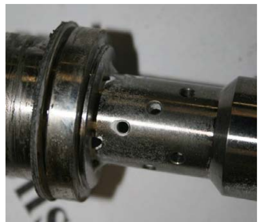
Modification of twin-fluid nozzle after 1 week of service and cleaning cycle.
