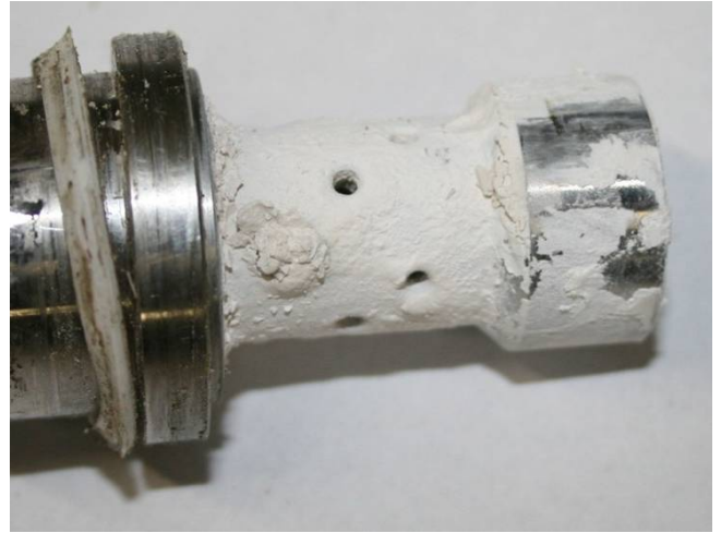
Fouling of twin-fluid nozzle spraying slurry after 1 week of service
