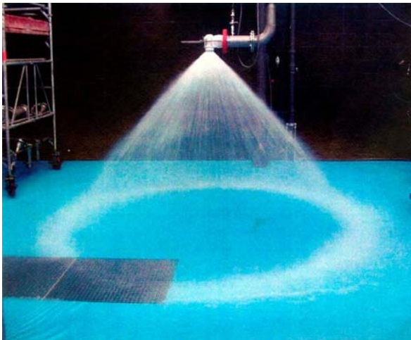
Large Single-fluid Hollowcone Nozzle used for Wet Flue Gas Desulphurization
