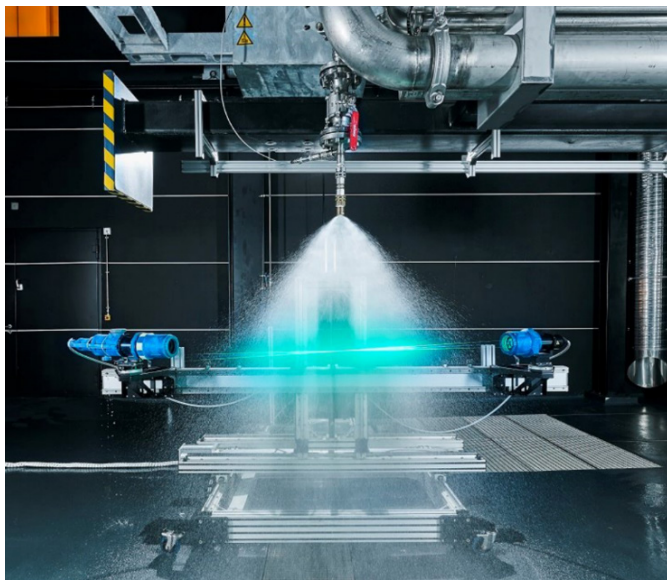
Figure 1 Image of traverse PDA spray plume analysis
