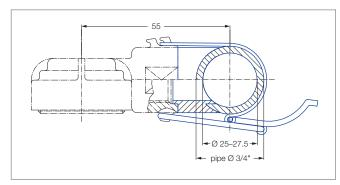
Recommended bore diameter 18 mm. Quick-release clamp unit: Ordering no. 035.030.15.05.00. Consisting of: Stainless steel clamp, polyurethane gasket.
