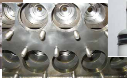
Stripped header after cleaning and pickling
