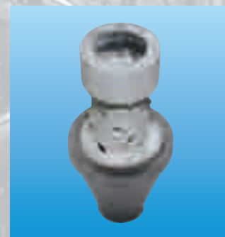
Nozzle blocked as a result of operation with lime slurry
