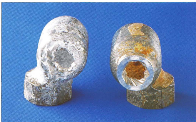
Alloy steel nozzles after about 300 operating hours
