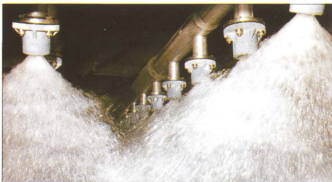
Full-cone nozzles in a flue-gas desulphurization plant
