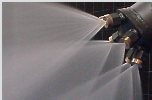
Cluster heads with 6 nozzles Operation at 35 bar
