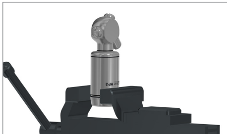
Clamping for undoing the second threaded joint
